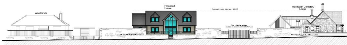
Figure 23 Street elevation depicting ridge height.
